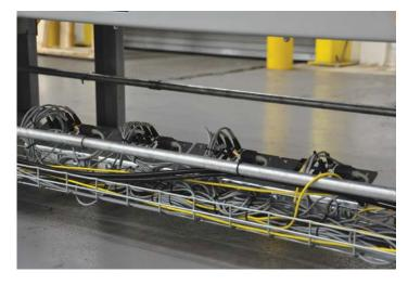
Machine wiring with SmartWire-DT
